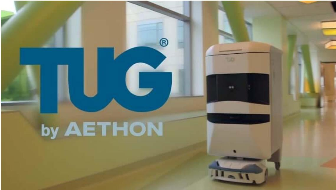
Aethon, founded in 2004 and based in Pittsburgh, is best known for its [TUG autonomous mobile delivery robot](#) which is able to carry around a multitude of racks, carts or bins up to 453 kilograms in the form of medications, laboratory specimens or other sensitive materials.
