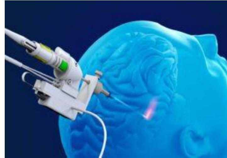
Minnetonka, Minnesota-based Monteris designed its NeuroBlate minimally invasive surgical robot system for controlled laser thermotherapy, known as laser interstitial thermal therapy (LITT).
