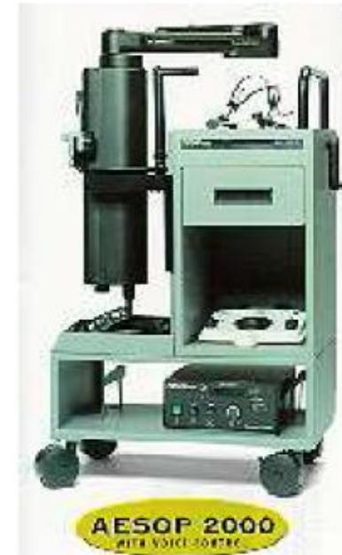
In 2001, the first robotic assistant **AESOP** (Automated Endoscopic System for Optimal Positioning) was imported from the United States to this clinic, used to hold an endoscopic camera and support minimally invasive surgeries. It was the first medical robot in Eastern Europe that served as an automatic assistant, among others. in coronary artery bypass surgery (by-pass) for over 300 operations.
